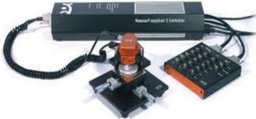
**Figura 3.10:** microscopio a forza atomica System "Nanosurf EasyScan2"
