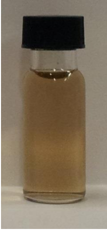
Figura 3.26: RuNPs ablate in i.PrOH, ns, 200 mJ, 14000 colpi
