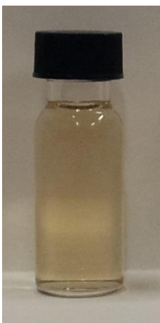
Figura 3.21: RuNPs ablate in i-PrOH, ns, 120 mJ, 14000 colpi
